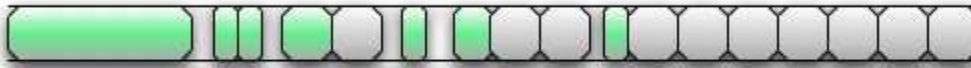
Figure 3: Defragmented heap with many allocations. We see a long line of same-sized buffers that we control.
